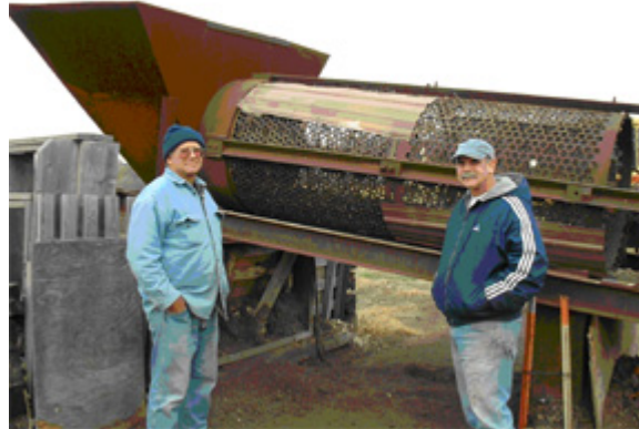
The finished compost runs through a sifter that sorts out the large composted materials.
